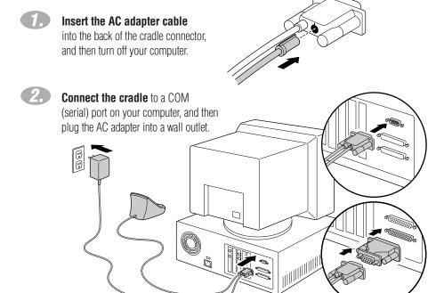
If necessary, use the included serial port adapter.
